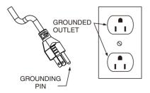
WARNING – Improper installation of the grounding plug is able to result in a risk of electric shock. When repair or replacement of the cord or plug is required, do not connect the grounding wire to either flat blade terminal. The wire with insulation having an outer surface that is green with or without yellow stripes is the grounding wire.
